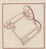
The speed of the motor is 1,425 R.P.M. which is, of course, much too fast for most of your machinery. To get down to the 60, 80 or 100 R.P.M. which you want, you will need a SPEED REDUCTION KIT. This Kit is portable also, and therefore, it is not essential to have more than one.
